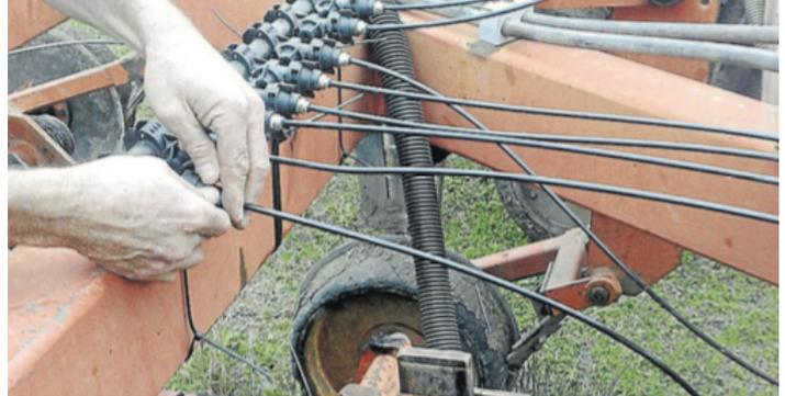
ABOVE: The Cordingley's planter, with liquid injection set up for Petrik application – in this instance it is set up for winter planting.
